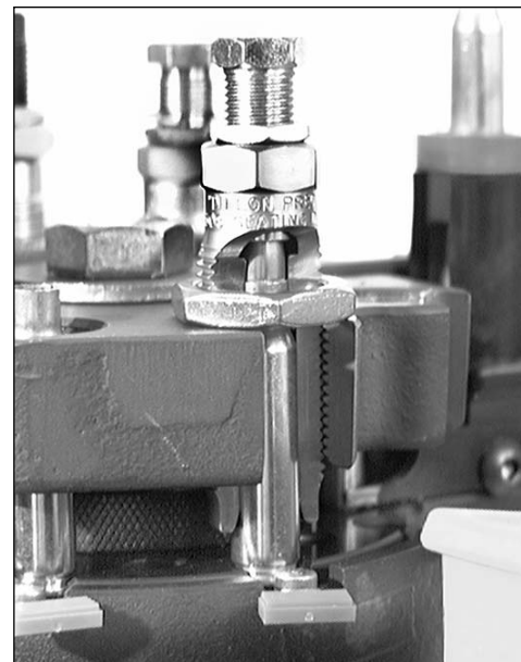
Station 7 - In this station, the bullet is seated to its proper depth.
