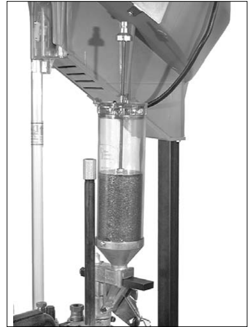
Fig. 25 - Dillon's Low Powder Sensor gives an audible and visual warning when the powder reservoir gets low.
