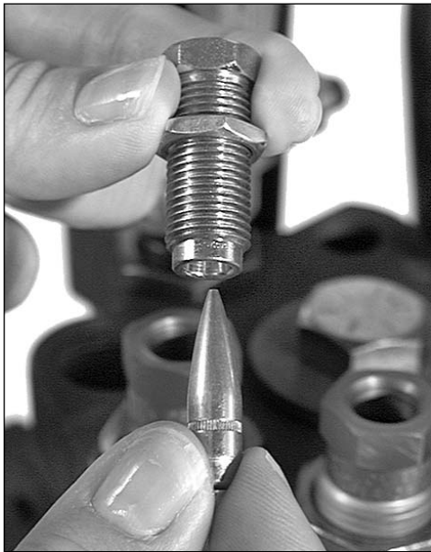
Fig. 56 - Place the bullet on the case mouth at Station 7.
