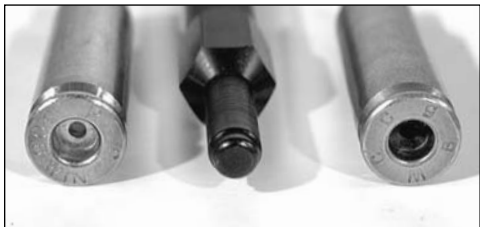
Fig. 32 - Note the difference between the swaged primer pocket (left) and the unswaged primer pocket (right).
