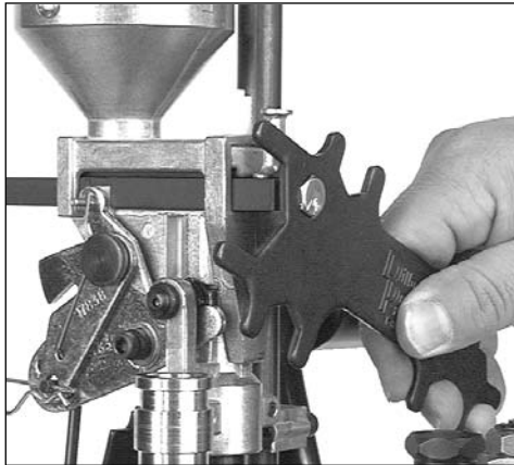
Fig. 19 - Clockwise turns of the powder bar adjustment bolt increase the powder charge while counterclockwise turns decrease the powder charge.
