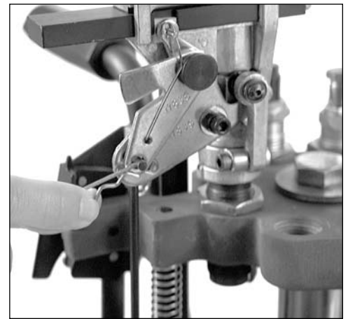
Fig. 42 - After removing the clip and disconnecting the rod, replace the clip in the rod for safe-keeping.
