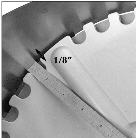
Fig. 27 - Make sure the casefeed plate is centered in the bowl with approximately 1/8" all the way around.
