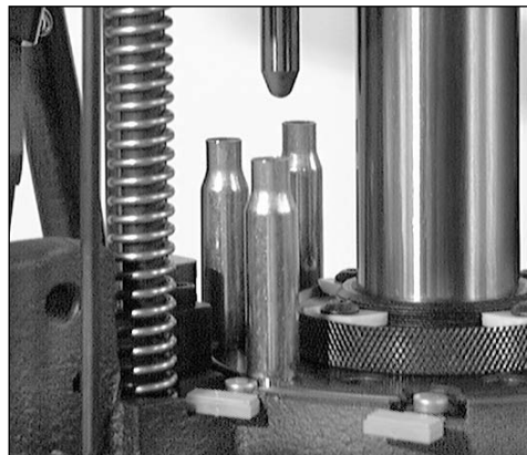
Station 5 - Here the case mouth is belled and powder dispensed.
