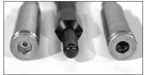
Fig. 29 - Note the difference between the swaged primer pocket (left) and the unswaged primer pocket (right).
