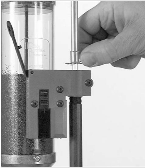
Fig. 22 - When installing primers into the primer magazine, be sure the pick-up tube centers itself before pulling the clip.
