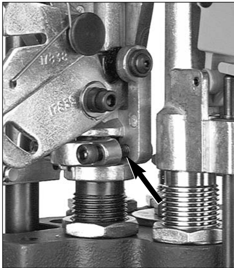
Fig. 9 - See arrow. A slight gap allows the powder die to be adjusted without removing the powder measure.
