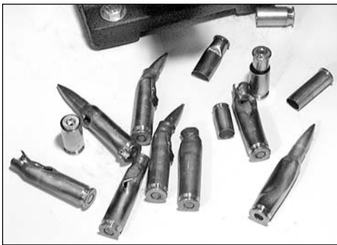
Fig. 23 - When loading, use only cleaned and inspected cartridge cases.
