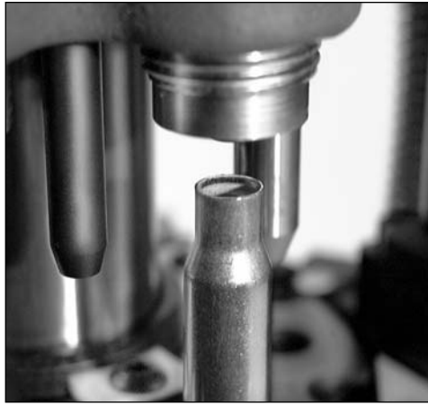
Fig. 49 - You don't need any more expansion than what you see in this photograph.
