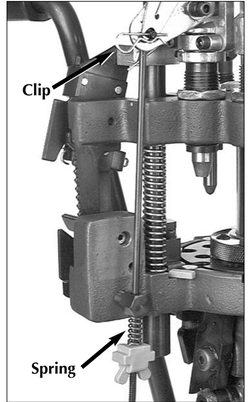
Fig. 10 - Note how the spring above the wing nut is slightly compressed.
