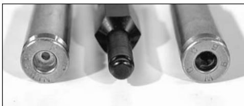
Fig. 58 - Note the difference between the swaged primer pocket (left) and the unswaged primer pocket (right).
