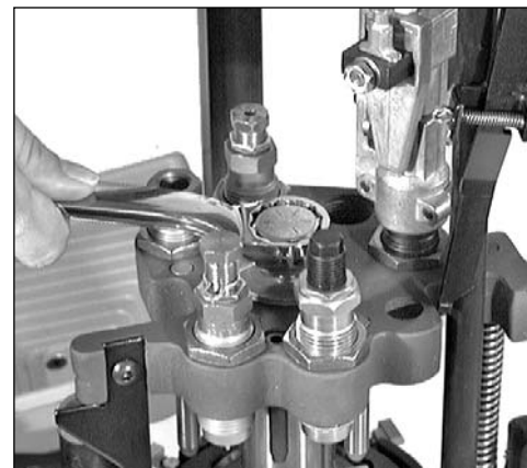
Fig. 36 - To remove the toolhead unscrew the toolhead bolt and remove.
