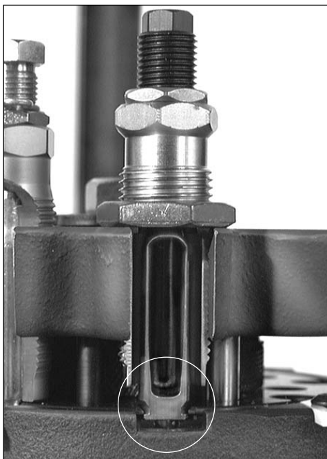
Station 3 - Here the case mouth is expanded while a rod supports the case base for swaging.
