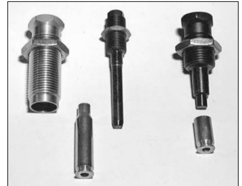
Fig. 15 - Note the difference between the rifle expander (center) and the pistol expander (right).
