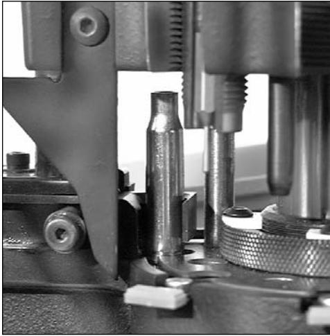
Station 1 - The casefeed plunger inserts the case into the shellplate.
