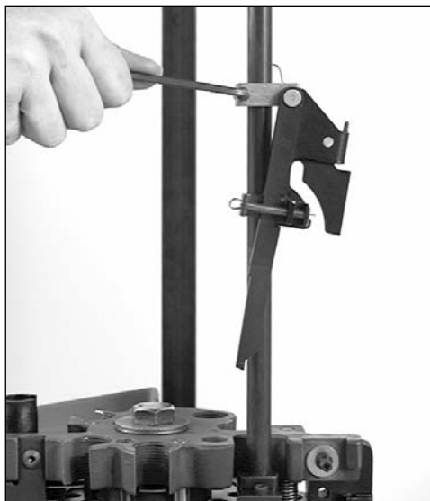
Fig. 34 - Slide the bracket assembly up and out of the way - retighten the lever arm bracket screw to hold it in place.
