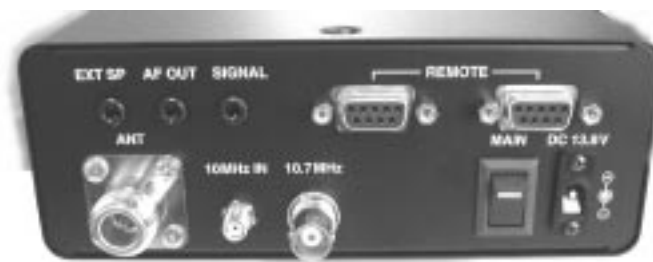
Main Power Switch ___ | ___ DC Power Jack
