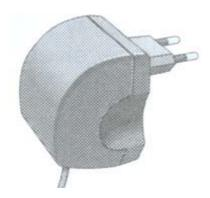
You can connect the set to the mains using a mains adapter. Only use a mains adapter, which supplies 4.5V DC with the negative pole at the center pin of the plug.
