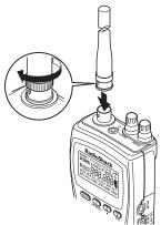
To attach the supplied flexible antenna to the connector on the top of your scanner, align the slots around the antenna's connector with the tabs on the scanner's BNC connector. Then slide the antenna's connector down over the scanner's connector and rotate the antenna connector's outer ring clockwise until it locks into place.
