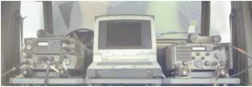
▲ HF/VHF communication node with the TRC 1731A multiservice terminal: E-mail, remote control, routing.
