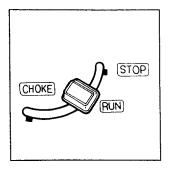
After 20 to 30 seconds of warm-up is completed, turn the engine switch to "RUN" position.
