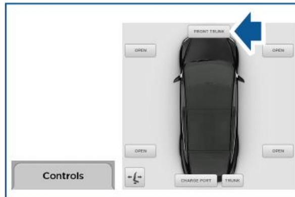
Figure 32. Opening the frunk using the touchscreen
