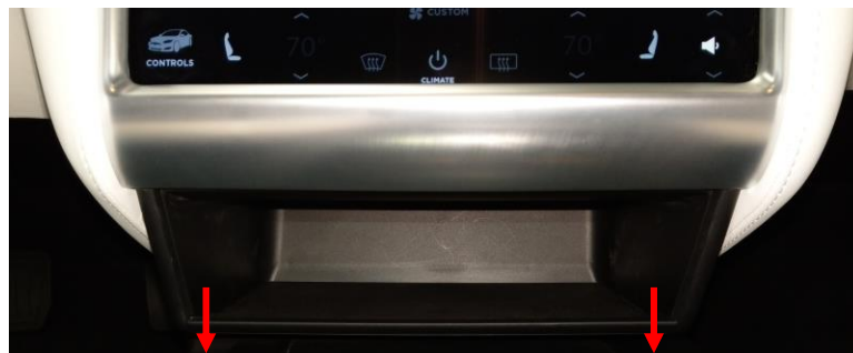
Figure 2. Releasing the storage pocket
