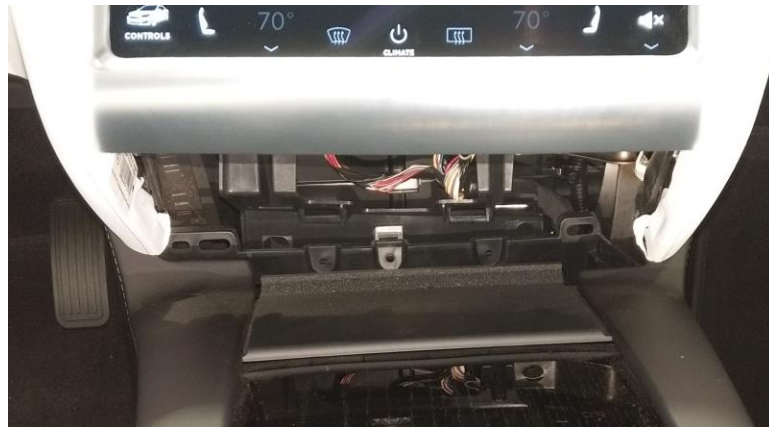
Figure 3. Removing the storage pocket
