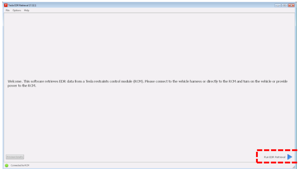
Figure 39. Retrieving data using the Tesla EDR retrieval program
