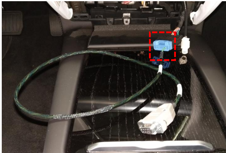
Figure 5. Moving the vehicle communication harness into position
