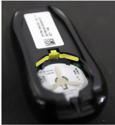
Figure 4 (Battery side terminal highlighted)
