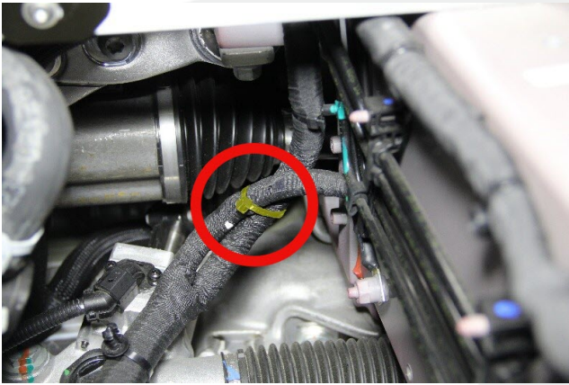
✓ Figure 1 – Cable tie highlighted
