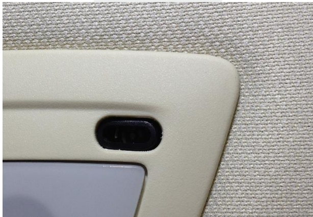
✗ Figure 2 (Sensor not flush with the map lamp assembly)
