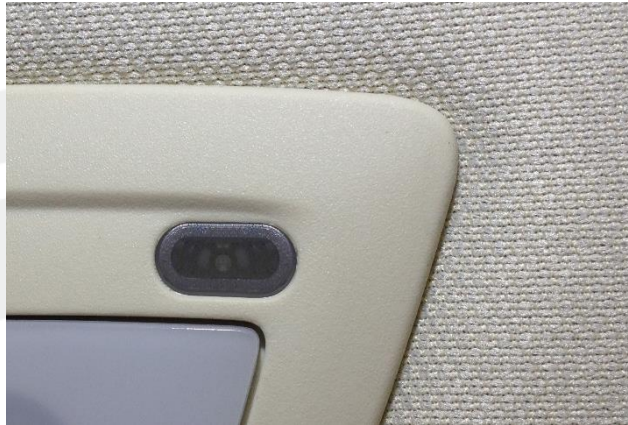
✓ Figure 1 (Sensor flush with the map lamp assembly)
