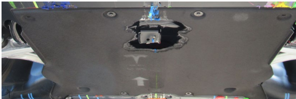
Figure 3 – Wear Through; Not Covered
