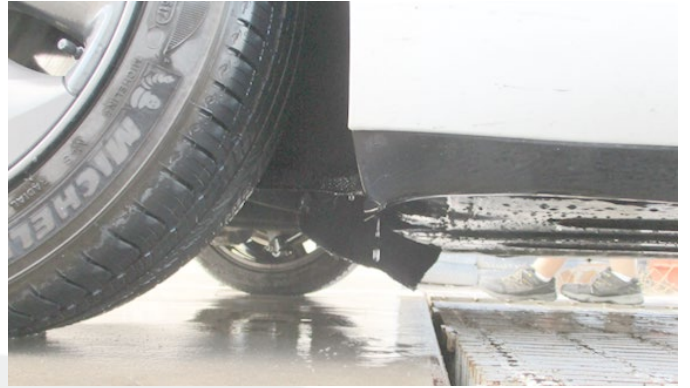
Figure 5 – Panel Folding at Leading Edge; Replace Panels
