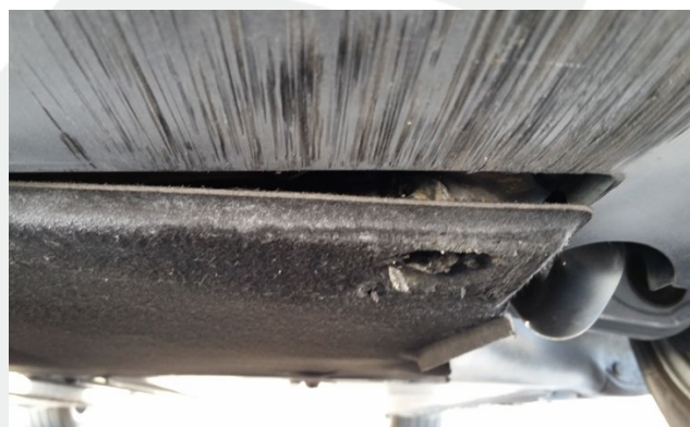
Figure 2 – Sheared Fasteners; Not Covered
