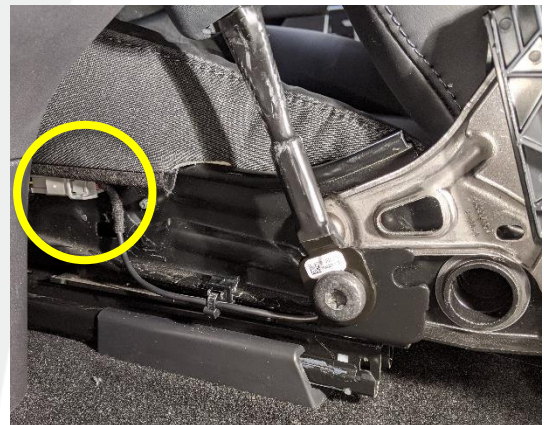
✓ Figure 5 – Buckle electrical harness attached to connector
