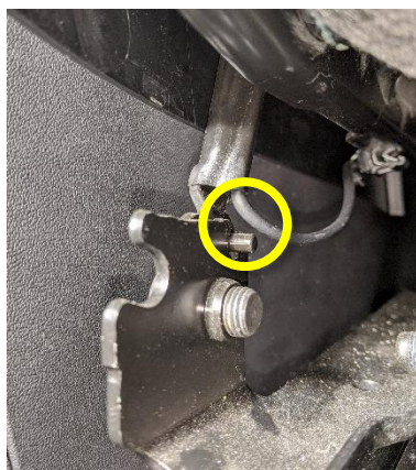
✓ Figure 11 – Harness in front of the seat recliner bolt and alignment pin
