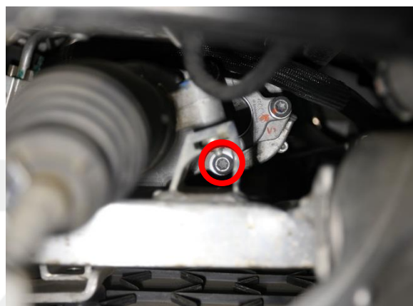
Figure 12 – Steering rack housing bolt 3
