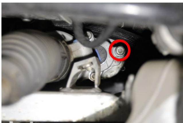
Figure 11 – Steering rack housing bolt 2
