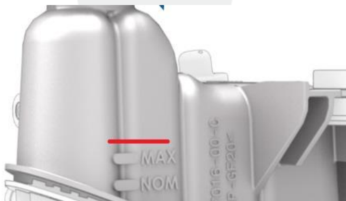
Figure 16 – Fill coolant to 5 mm above “Max” line
