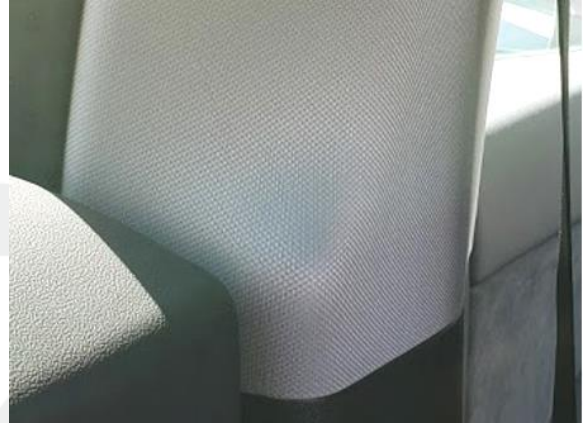
✔ Figure 2 – No casting seam
