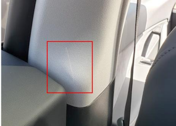
✘ Figure 1 – Casting seam
