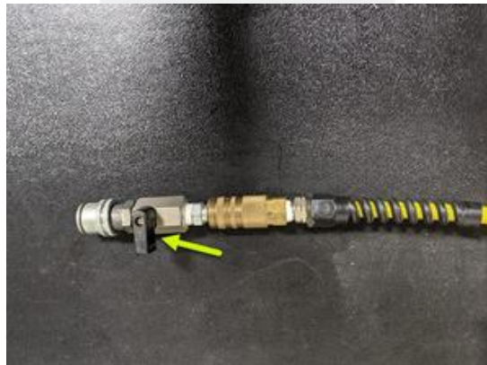
Figure 9 – Air Line Valve
