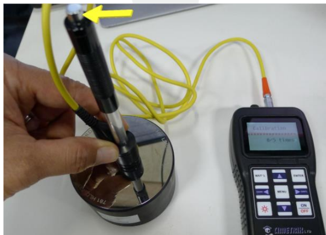
Figure 2 – Press the release button to trigger the impact tool
