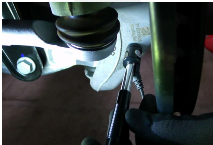
Figure 13 – Striking location on the LH front knuckle
