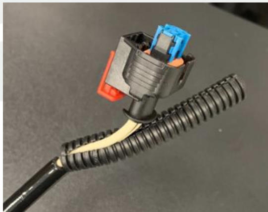
Figure 9 – EPB electrical connector disconnected for clarity
