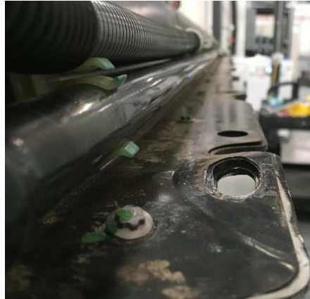
Figure 12 – Deburr the area to remove sharp edges
