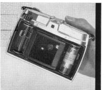
Place a roll of fresh Ansco film into the righthand chamber by pressing it against the spring and sliding it into the curved spool holders. Be sure the printed side of the film's backing paper faces you when the film is unrolled.
