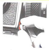
B. Safety Lock The shutter release button has three settings to which it can be set by rotating in the clockwise direction. Two of these settings have safety locking features of slight difference. The three positions are indicated by the red dot being placed at the bottom, at a position 45° from bottom setting and at the side. with functions differing as per table
