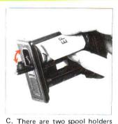
on the film holder. The top one is for the fresh film spool while the bottom one is for the empty take-up spool. The left-side shafts of both spool holders can be opened outwards, as illustrated. Therefore, insert the right end of the spool on to the right-side shaft, which is fixed, and then close the left-side holder (shaft) which will engage the spool.
