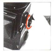
H. Upon loading the film, rotate the film winding crank until it stops to place the first frame into place for taking the picture. The exposure counter will also change from "S" to "1", while the shutter will also be cocked.
