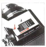
B. Depress the battery chamber button with your finger and, at the same time, move the battery chamber cover in the arrow-indicated direction. The cover will come off easily.
