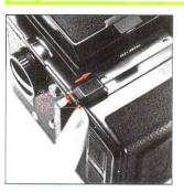
A. To detach the film holder. open the back cover. First, press the safety lock (1) in the arrow-indicated direction and then push the back cover release button (2) towards the exposure counter.
