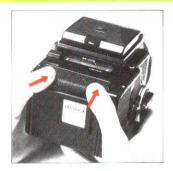
G. Close the back cover, by pressing it firmly against the base of the film back, as illustrated. The back cover will automatically lock and close, with the safety lock also locking the back cover release button.
