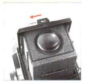
B. The magnifier can be flipped up into viewing position, by simply sliding the focusing hood/magnifier catch in the arrowindicated direction (to the left). To return the magnifier to its storage position, simply push it down until it catches.
