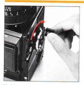
H. Upon loading the film, rotate the film winding crank until it stops to place the first frame into place for taking the picture. The exposure counter will also change from "S" to "1", while the shutter will also be cocked
