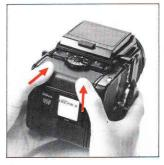
G. Close the back cover, by pressing it firmly against the base of the film back, as illustrated. The back cover will automatically lock and close.
