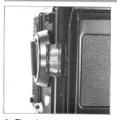
A. The shutter speed scale is viewed in its window over the shutter speed dial. The numbers on the scale are shutter speed settings, with numbers 1 to 8S full numbers and numbers 2 to 500 fractions of a second. For example, "8S" is 8 sec., "2S" is 2 sec. and "500" is 1/500 sec. \* The shutter is released at 1/500 sec., regardless of the setting when the battery is not loaded or is completely drained.
