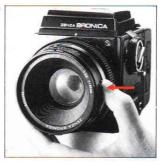
B. All interchangeable lenses for the Zenza Bronica SQ have fully automatic lens diaphragms which means that the focusing screen is always viewed at the full aperture, with the brightest possible image. However, depressing the depth of field preview lever will stop the lens diaphragm down to the pre-selected lens opening and permit the photographer to check the depth of field effect on the focusing screen.
