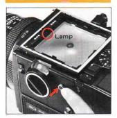
If a red-colored LED battery check lamp lights up outside the focusing screen area (central front of finder), when the battery check lamp is pressed, the battery is loaded properly and there is sufficient power for operations.
