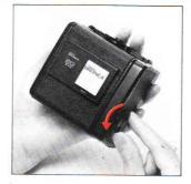
When the film back is detached from the camera body for film loading, the manual film winder is used for advancing the film. The film will stop when it is in place for the first exposure, with the exposure counter also changing to "1". However, it will be possible to rotate the manual film winder and, therefore, it should be rotated 2 or 3 times more, in order to take up any slack in the loaded film.
