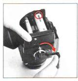
F. The starting point, or arrow mark, can also be aligned with the start-mark, with the film holder loaded in the film back. Simply rotate the film winding crank on the camera body, in this case. This method is preferred since there will be coupling with the camera body mechanism, from the beginning.
