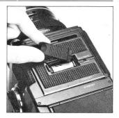
B. Coincide the plus (+) and minus (-) marks on the battery with similar polarity indications in the battery chamber. Then, push in the battery.
