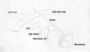
produced by the light cell when the meter pointer is at full-scale position.
