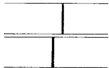
As image will appear when Range Finder is set for a distance nearer than the correct one.
