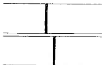
As image will appear when Range Finder is set for a distance beyond the correct one.
