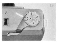
(ASA) adjustment, turn the exposure control until the filmspeed indication shows the ASA rating of the film you are using.
