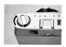
Turn the fillm counter clockwise to bring "S" (start) into alignment with the index mark. Take three shots with lens cap on to bring film counter to "l" where picture-taking can be started.
