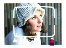
18 To make exposures, hold camera steady against your face with both hands and push the shutter release button with a slow, gentle squeeze. This is particularly important when the red warning appears in the viewfinder when the shutter is set at 1/30 sec.
