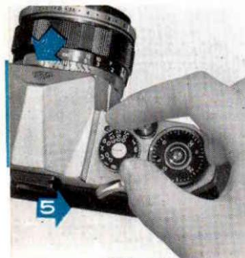
6. Cock the automatic diaphragm lever for full-aperture viewing.
