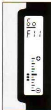
**3. Change the shutter speed by moving the select switch or the aperture by moving the select switch while holding down the exposure compensation button.**
