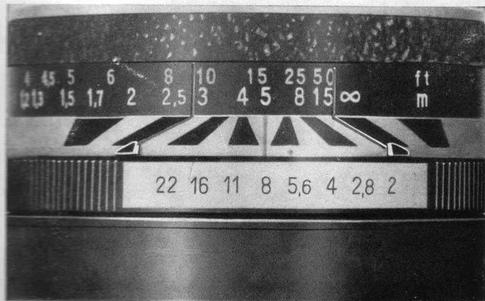
Distance 5 m (15 ft.) Aperture f/8 Depth of field from 3 m to 15 m (10 ft. to 50 ft.)
