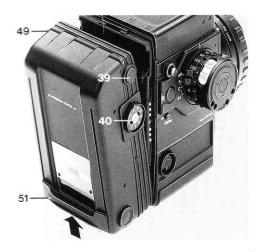
abunter window 53). This opens the laminar drawslide and secures the magazine on the camera. It also unblocks the metering and exposure functions.
