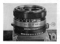
lengths are longer in wave lengths and not visible to the naked eye. The infrared index (10) is the red line representing f/4 opening on the depth of scale, which should be used for making such adjustments.
