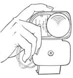
For incident light readings fit the Invercone as shown on page 5 and hold the meter as shown here; use the index finger to operate the pointer lock.
