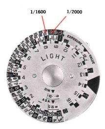
If it is desired to shoot at shutter speeds faster than the 1/1200 second indicated on the meter dial, or at an aperture above f/32, these ranges can be extended in the following manner.
