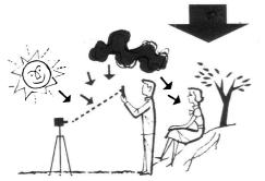
Reflected light is light reflected from the subject to the camera. Incident light is the light which falls on the subject. Measurement of either reflected or incident light can be used to determine correct exposure.
