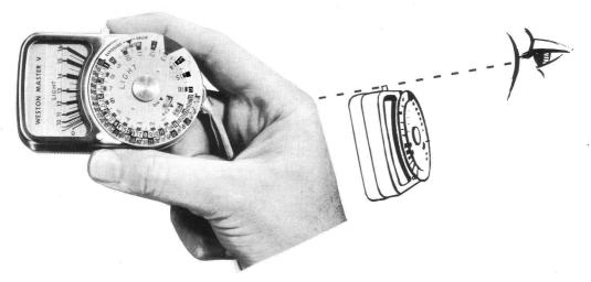
The best way to hold the meter is shown in the illustration. Be careful not to obstruct the photocell with your fingers or have the neckcord dangling across the cell opening. In outdoor general scenes, when the reading is taken from the camera position, tilt the meter at an angle slightly downward so that your line of sight passes over the front edge of the pointer lock, as shown in the insert. This will exclude sky areas which would tend to inflate the reading and cause underexposure.
