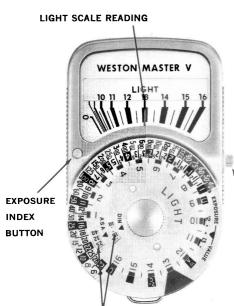
SET THE FILM EXPOSURE INDEX by first depressing the EXPOSURE INDEX BUTTON, then rotate the dial until the desired exposure index number appears in the window. Release button and the EXPOSURE INDEX locks into place. The Exposure Index number (commonly called "ASA Index") is given on the film manufacturer's data sheet enclosed with the film. For example let's assume an Exposure Index number of 32 (See illustration).
