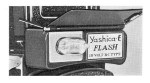
Press the Flash Cover Release Button and the cover will snap open. Push a new AG-1 bulb into the socket. You are now ready to shoot.
