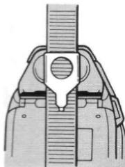
If you remove your eye from the viewfinder eyepiece during focusing (when taking pictures with the self-timer, for example), attach the Eyepiece Cover as shown.
