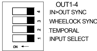
Figure 4: Output DIP Switch(s)
