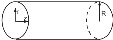
FIGURE 5.9 One-dimensional heat transfer in a cylinder in the r direction. Common boundary conditions are (1) constant wall temperature at r = R and a zero heat flux in the r direction at the center (i.e., q_r = 0 ); and (2) heat flux at r = R due to thermal resistance between a fluid and the cylinder surface.
