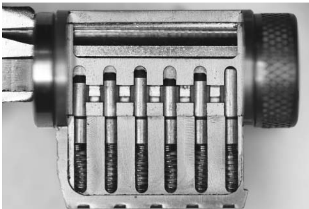
Figure 11.1: A cutaway pin-tumbler lock (Courtesy of Marc Weber Tobias)
