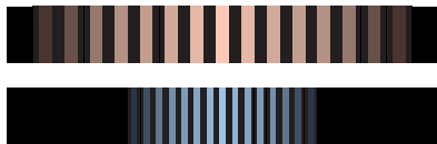
(g) Double-slit diffraction patterns of long-wavelength red light (top) and short-wavelength blue light (bottom).
