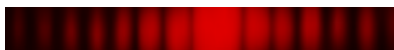
(b) Single-slit diffraction of red light. Note the double width of the central maximum. (Photo by the author.)
