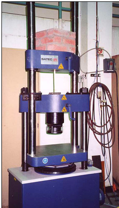
Fig 14.10: Brick sample loaded in tester
