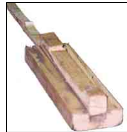
Fig 14.4: Epoxy glued support end
