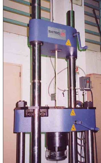
Fig 14.6: Specimen with no supports loaded in tester
