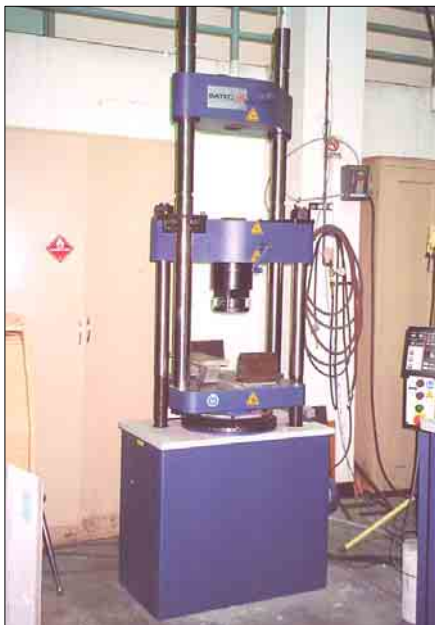
Fig 15.1: 5590 HVL series Universal tester and computer for operation
