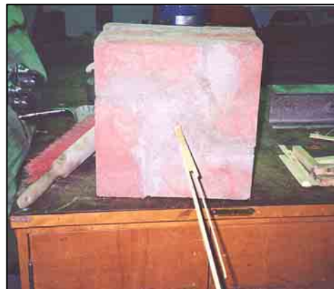
Fig 14.11: Brick with embedded splint
