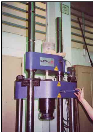
Fig 14.8: Mortar sample loaded in tester
