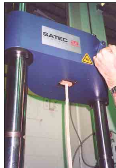
Fig 14.2: Specimen loaded in tester
