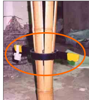
Fig 15.7: Bamboo Splitting method
