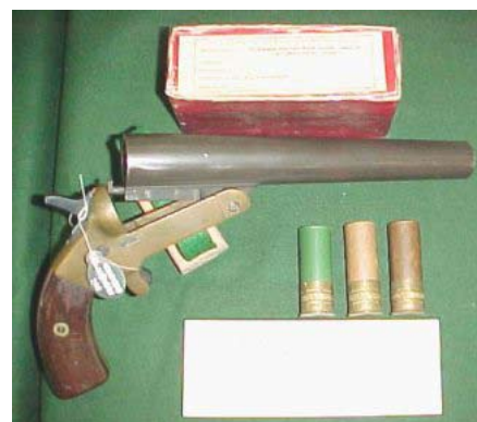
This "signal pistol" or flare gun is one of 20,000 made by Remington's Bridgeport Connecticut plant, along with the green, white and red flares for it.
