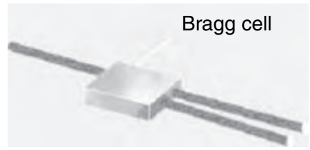
Figure 10.1.8. Bragg cell used as a beam splitter.
