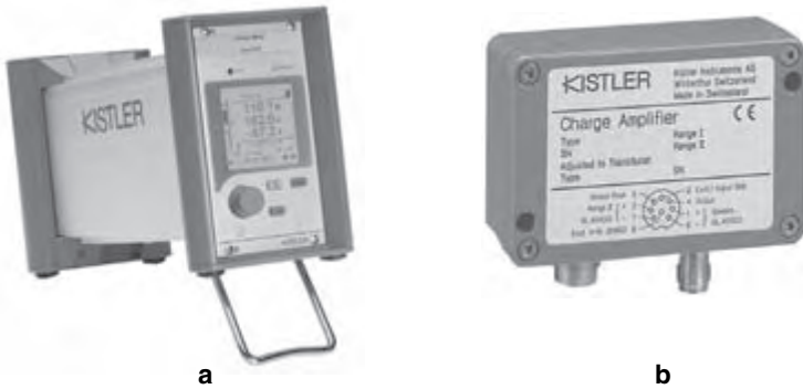
Figure 16.2.3a: Charge amplifier for laboratory applications. Virtually any type of sensors (including force sensors and accelerometers) with charge output can be connected to the input. Figure 16.2.3b: Industrial charge amplifier with two remotely switchable measuring ranges (courtesy of Kistler).
