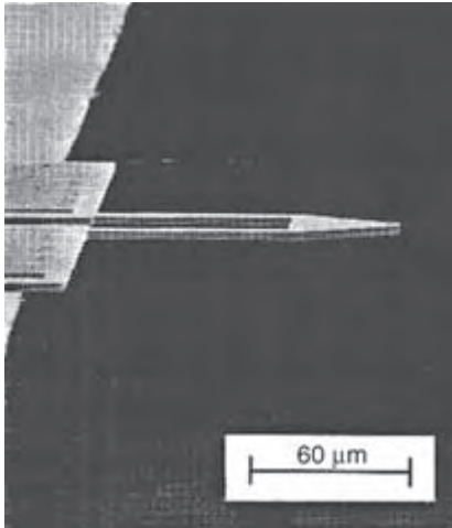
Figure 19.1.3: Silicon strain gage. (Dr. Marco Tortonese, PhD thesis, Stanford University, 1992.)
