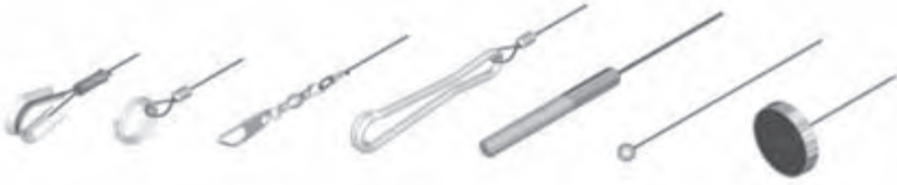
Figure 15.2.3: A few displacement cable terminations.
