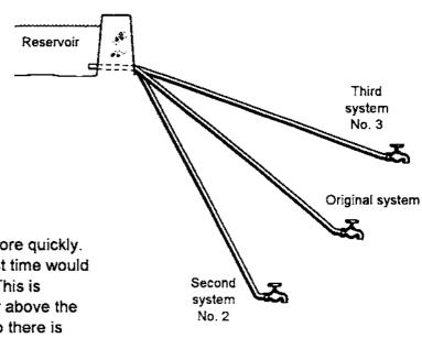
As the water gets faster the friction between it and the wall of the pipe gets greater. The curve of the line on the graph begins to flatten out. When the water is flowing as fast as it can, the line on the graph is flat. Because the *head* in the second system is greater than the *head* in the first, the water flows faster in the second. This is shown on the graph at the top of the next page.
