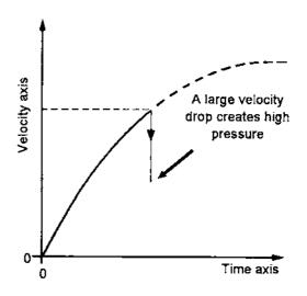
When the *delivery head* is small, the velocity only has to drop a small amount before the pressure in the pump is higher than the pressure in the air vessel.
