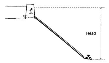
When the tap is opened, water starts to flow down the pipe and out through it. It flows slowly at first, but speeds up very quickly. After a short time the water reaches its maximum speed and the flow becomes steady. If the tap is left open, water will of course continue to flow steadily down the pipe from the reservoir and out through the open tap.
