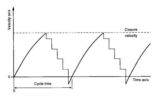
The impulse valve closes and the pump beats every time the line on the graph reaches closure velocity. For a pump working at 60 cycles a minute, the "cycle time" would be 1 second.
