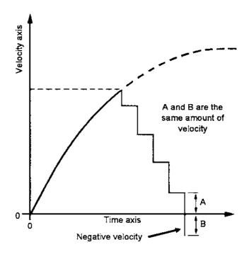
As the water moves away from the pump it has a negative velocity, so the line on the graph goes under the base (under 0 on the Velocity axis). The negative velocity will be the same size as the positive velocity that was left when the delivery valve closed. When the water has a negative velocity it moves away from the pump towards the drive tank.
