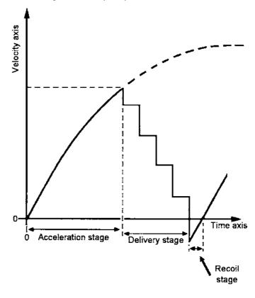
When the water has stopped recoiling, it starts to flow down the drive pipe and out through the open impulse valve again. It accelerates down the drive pipe and through the open valve as it did at the start of the pumping cycle.
