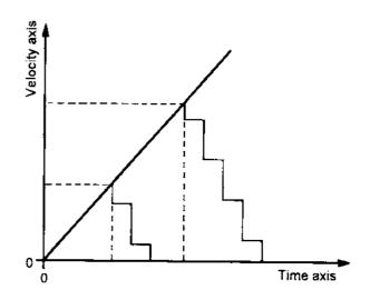
If the impulse valve was tuned so that the stroke was very long or the weight very heavy, the closure velocity would be in the flatter section of the line on the graph. The drive flow through the pump would increase a lot but the delivery flow would change very little. The time taken for each cycle would also increase so that there would be fewer cycles per minute. The pump would become less efficient and would actually pump less water per minute.
