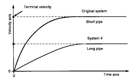
On the graph of this example above, the original system is also shown. The line on the graph flattens out at a lower speed and in a longer time.
