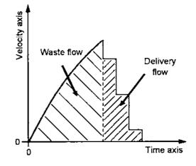
When the area under the falling part of the graph is large it means that there is a large delivery flow. Two things increase this area. One is increasing its height. The other is increasing its width either by having more steps or by having longer steps.
