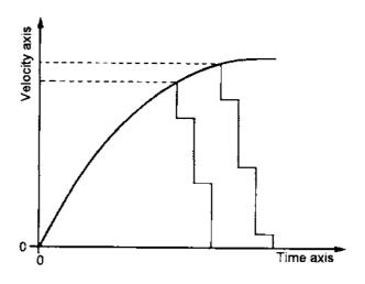
Increasing the weight and stroke of the impulse valve too much would stop the valve from closing at all. This is because the valve cannot close when the velocity needed to close it is more than the terminal velocity of the water through the pipe.
