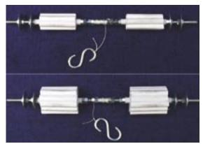
4. This is how a slow shaft should look like – use the short threaded rod. The two big washers at both ends of the shaft will keep the shaft in place. They are fixed using two nuts each. The gear wheels are also fixed with nuts. One end of the string is squeezed in between two nuts, the other one is attached
