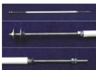
4. As you want the rotor to turn smoothly, the shaft (threaded rod) must run in a bearing. Use two sheets of A4 paper (landscape format) to roll a rigid tube with the wooden stick. Put the shaft through the tube (top picture). On the left end you can mount the sail rotor (centre), on the right end you may squeeze a string between the two nuts for lifting objects with the rotor. Place a cork or rounded plastic button on the protruding end of the shaft for safety.
