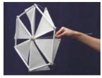
**3.** Put the threaded rod through the rotor's centre hole and fix the rotor using a big washer and a nut on either side. Use a wrench (spanner) to tighten the nuts. The sails are fixed to the rotor lattice using cable ties (centre), bolts, and strings (edge). You can simply sling the string around the nearest bolt and make a knot.
