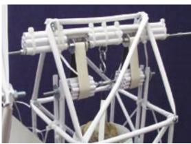
8. If you use this setup, you will be able to lift really heavy loads. Hang the slow shaft with the big gear wheels (transmission ratio of 1:5) into the belts. Do not attach the hook directly to the load, but sling it around the handle and attach it to the ring mounted in the center of the beam. With this socalled
