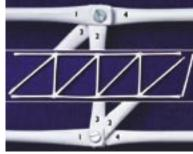
**5.** Put the bars together to form a lattice, as shown in the centre image: the 12 short bars are used for the edges, the 4 long ones for the diagonals. A node is made by placing bars no. 1-4 on top of each other. Insert the bolt through the holes of each of the bars. (Note: The order of bars is different for top and bottom nodes!) Finally, put a washer and a nut on the bolt and tighten it with a screwdriver.
