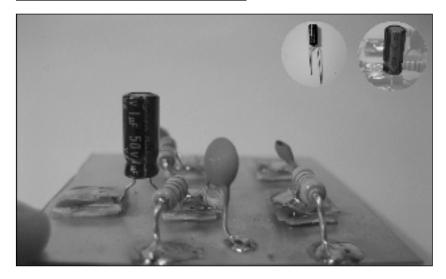
The polarized capacitor is special. This one does need to be soldered on the right way round.
