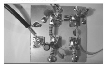
So now you're almost done with the building part. As you will understand, the antenna makes the signal go further. It does not help to make this thing as long as possible, actually every frequency has a preferred antenna length. Which I'll discuss later.
