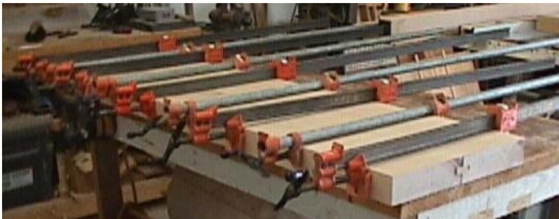
Top slab being glued up. Notice the plywood spline to help in alignment.
