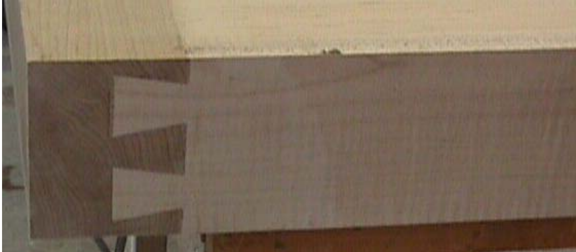
The dovetails on the back apron and back of the end caps.
