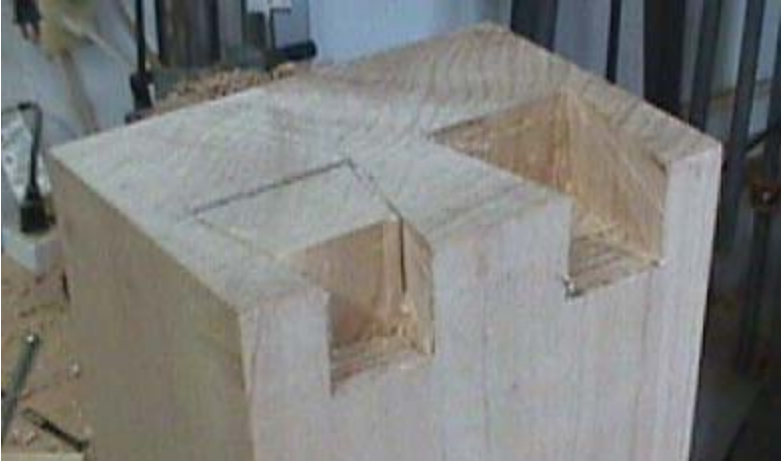
The half blind dovetail pins being cut on the end caps.
