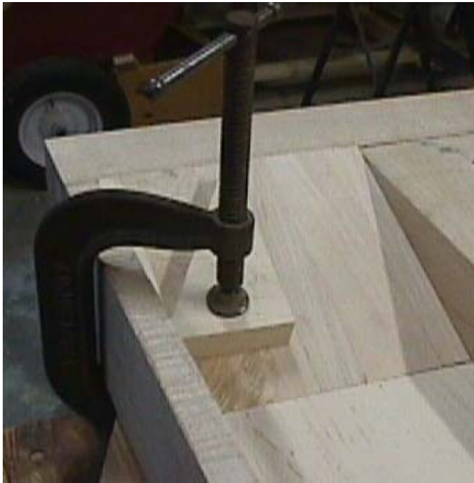
Clamping the ramp into place as it is glued.
