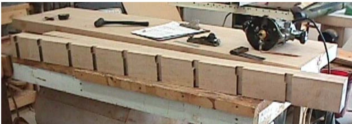
The finished dog-holes.
