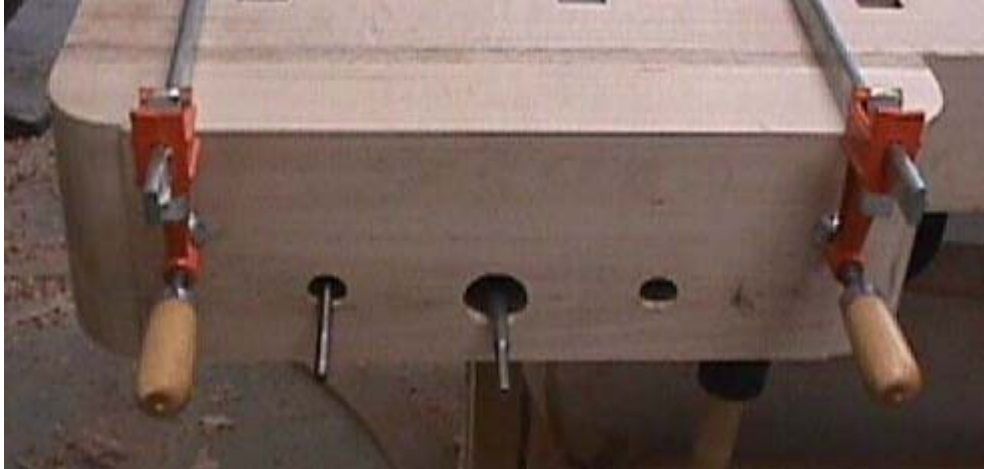
Using drill bits to mark the center of holes on the bench.
