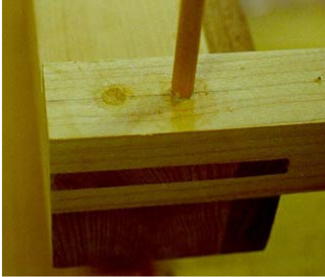
Pinning the finger joint with dowels
