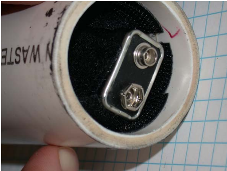
Covering battery in Velcro and then securing it in the piping.
