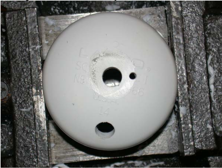
Drilling the holes in the end cap
