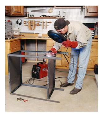
**Attach the remaining legs.** Repeat the instructions on attaching the leg in step 5. Check to make sure you completed all welds on both sides of each leg before standing the table on its own weight.
