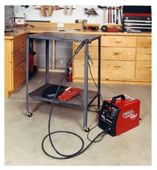
Stand back, admire your handiwork and start on your next welding project. You may want to paint the welding table with a rust-resistant paint, but DO NOT PAINT THE TOP OF THE TABLE. You will want this to remain bare steel so metal parts placed on the tabletop for welding are in contact with the work. Before painting, clean the entire table with a cleaning solvent to remove machining oils. Mask off the top with masking tape and newspaper. Paint.
