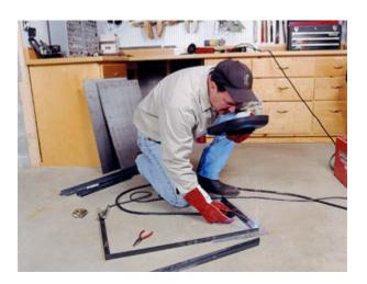
Welding the two frames for the tabletop and shelf. Using the square on the outer edge, place one piece of 30-inch angle iron and one piece of 18-inch angle iron together, mitered side down, making sure they are perfectly square.
