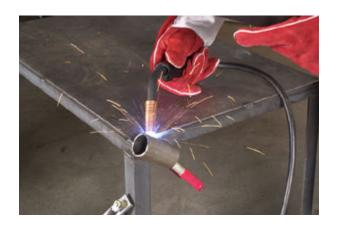
Attach the welding gun holder. With a clamp, attach the 3-inch length of steel tubing to the right front corner of the top shelf of the table (if right-handed; be sure to switch to the left side if you are left-handed). Attach it at approximately a 45-degree angle with the front facing up to accommodate holding the gun (see photo). Tack weld the tube and remove the clamp. Make a 1-inch finish weld on the topside of the tube.
