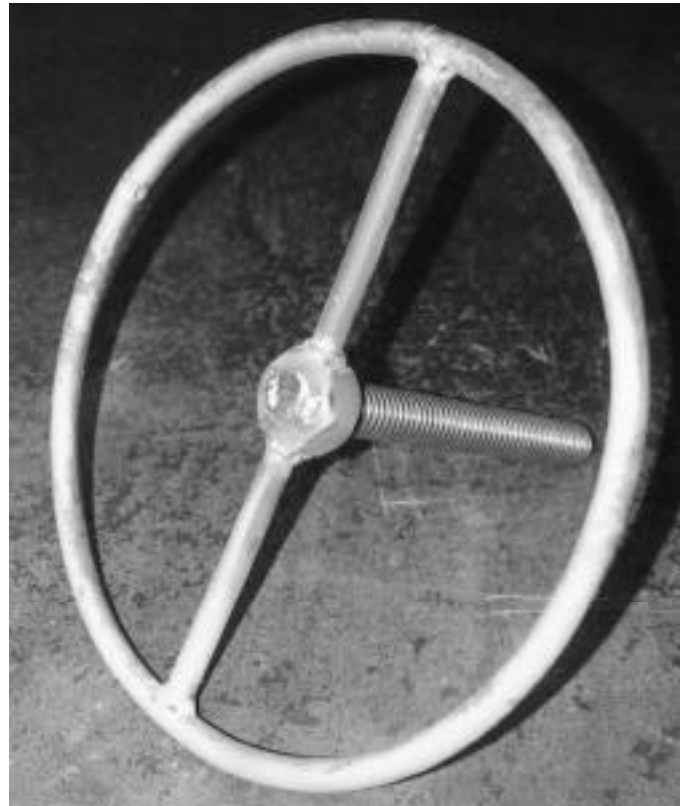
The handwheel fabrication
