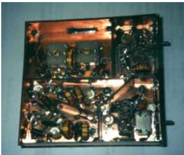
This module contains converters for 160 meters and 17 meters.
