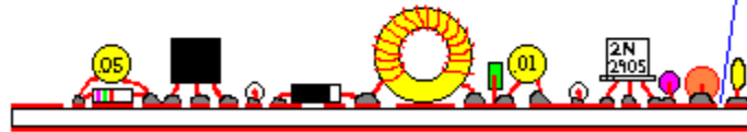
"Gouged Board" - Parts soldered to islands and traces on 2-sided p.c. board.
